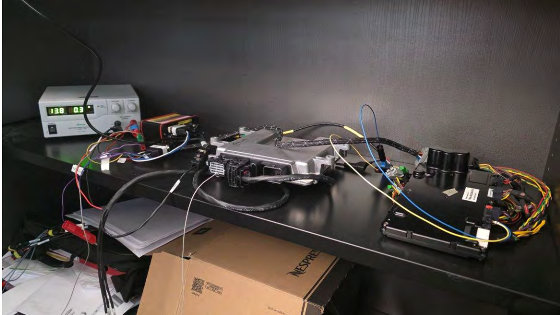
Figure 3-8: vHIL setup: starting from the left: 12V power supply, CAN device, DANA Pinnovo, SBMS.
